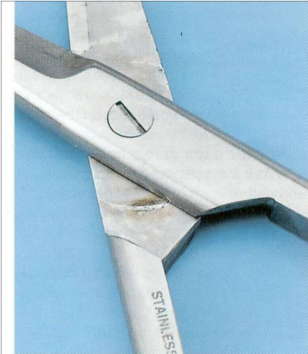
Fretting corrosion due to insufficient lubrication
